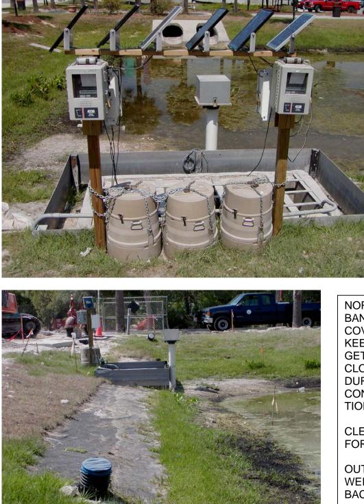
SAMPLING EQUIPMENT FOR DETAILED STUDY SHOWING FLOW METERS AND SAMPLERS AT OUTFLOW
