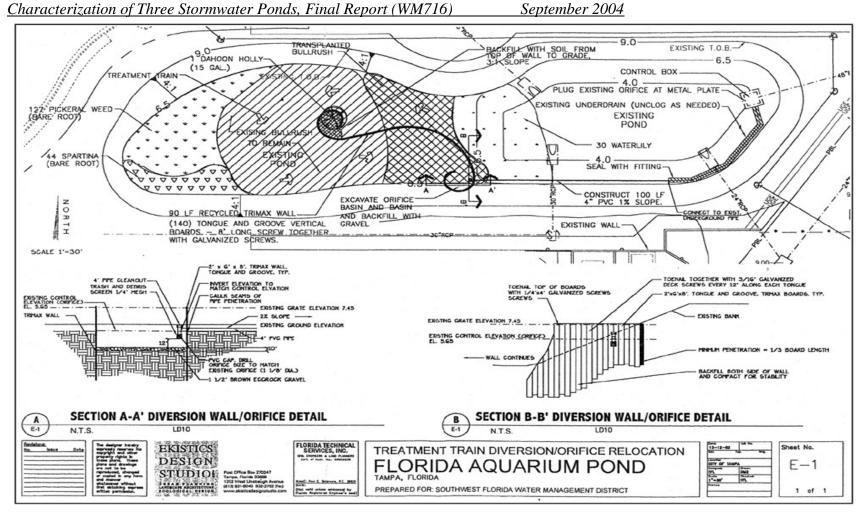
Figure 29. The site plan shows the alterations to the Building pond with the diversion structure and new plantings. Also note the three inflow pipes close to the control box (outflow weir).
