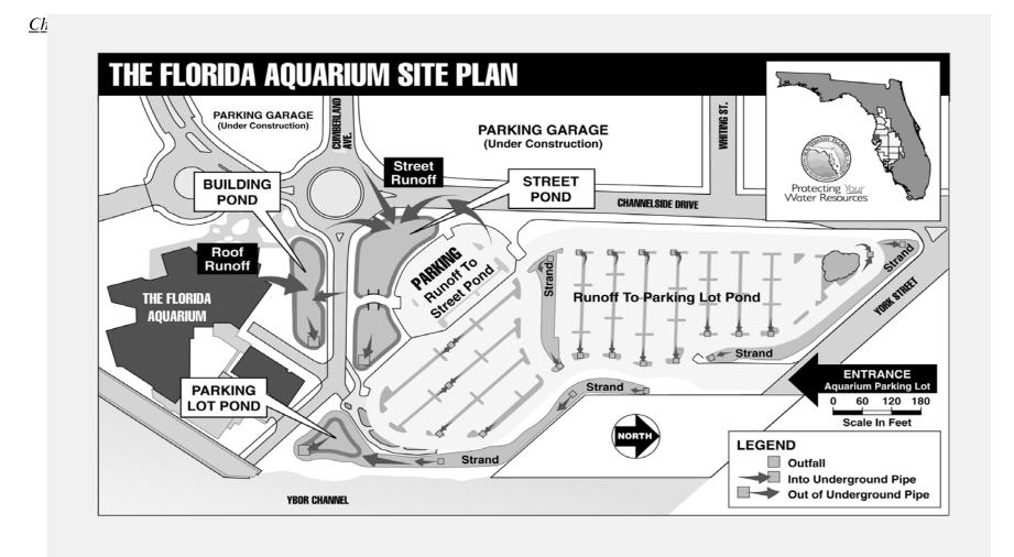
Figure 1a. Site plan showing the three stormwater ponds and the layout of the whole basin stormwater system used for he Parking Lot Pond.
