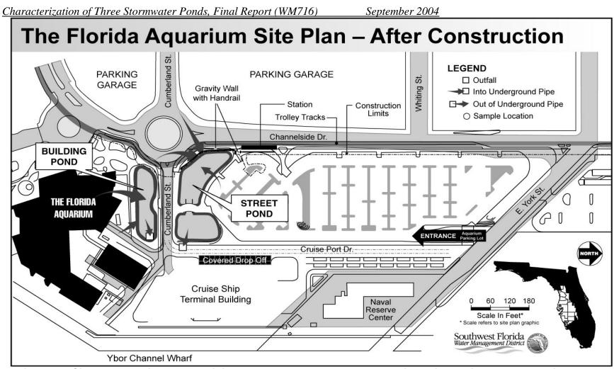
Figure 1b. Site plan showing the remaining two stormwater ponds, new cruise ship terminal, the trolley line and the layout of the basin after the construction activity.
