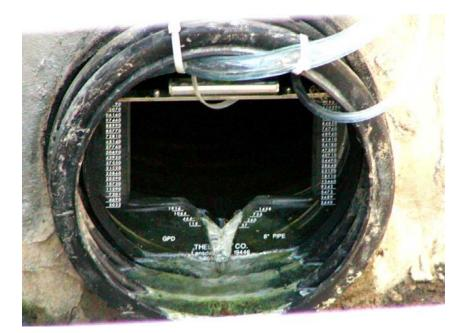
UNDER DRAIN PIPE WITH THELMAR WEIR MEASURING DEVICE
