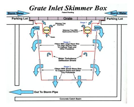
Figure J-1. Diagram of drop box insert.
