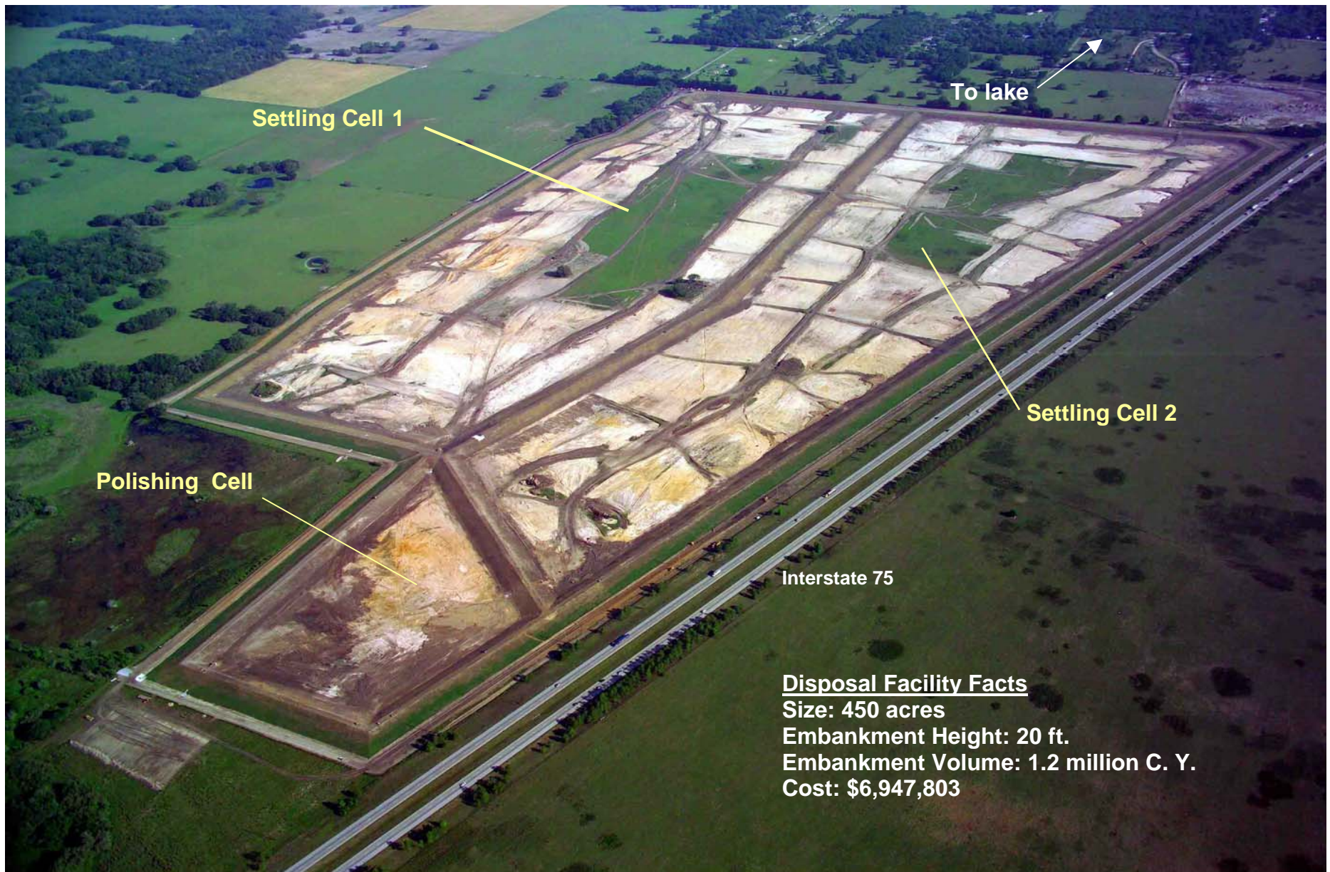
Lake Panasoffkee Restoration Project – Upland Confined Disposal Facility for Steps 2 and 3 (Oblique View Looking Northwest)
